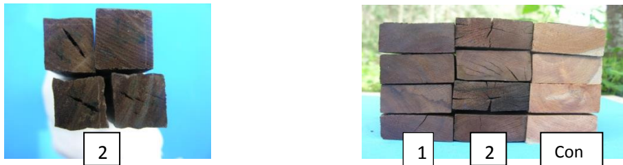
Figure 1 Defects on wood specimens from treating with different heating condition ; kiln-drying (condition 1) , high stream or auto cleave (condition 2) and no- treatment (control).
